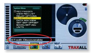
A "BTooth Discoverable" prompt means that TRAXALL Bluetooth is active, but it is still necessary to establish communication with your PC or laptop and then launch the TRAXALL Remote Control application. (See following pages.)
