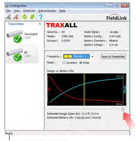
A fixed yellow line near the center of the range-power graph indicates the estimated optimal balance for the selected transmitter. As you move the slider to this line it will momentarily "snap" in place.
