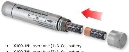
X100-2N: Insert two (2) N-Cell batteries
