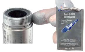
Screw battery cap onto transmitter.
