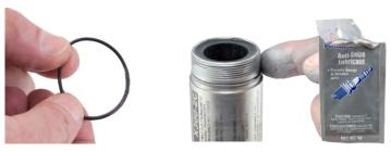
Carefully lower the end cap over the flexible antenna circuitry until cap and transmitter screw threads meet.
