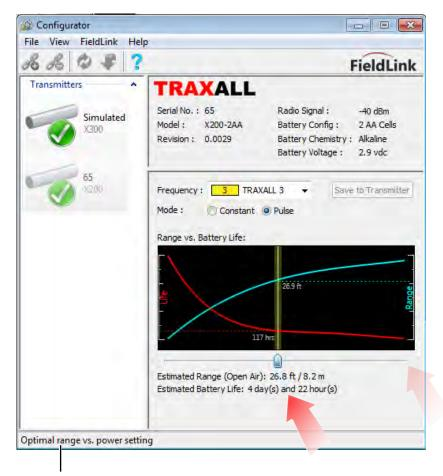
STATUS: OPTIMAL RANGE/POWER BALANCE FOR THIS TRANSMITTER
