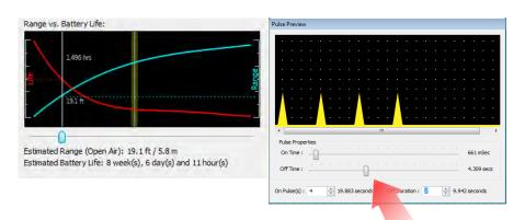
Further decreasing Range, decreasing On Pulses, and increasing Off Duration can extend this transmitter's run time beyond 40 weeks!
