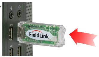
A red LED on the device will flash every three seconds, indicating Configurator is seeking to establish a communication link with a transmitter.
