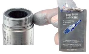
Screw battery cap onto transmitter.
