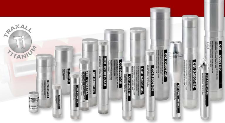
**CDI X-SERIES TITANIUM TRANSMITTERS** are TRAXALL-compatible electromagnetic pipeline pig-tracking devices specially designed and titanium constructed for high-pressure (7,500 psi/517 bar) pipeline environments. Like our standard stainless steel transmitters, they offer both programmable frequency and power control through CDI's proprietary FieldLink wireless communications system.
