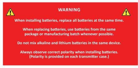
**EX EX NOTE** for ATEX/IECEx applications: DURACELL® PROCELL alkaline batteries or Electrochem lithium batteries are required by ATEX and/or IECEx standards to maintain system certification.
