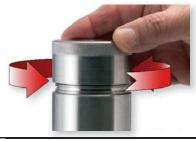
Screw antenna end cap onto transmitter. Do not over torque. Hand tightening is sufficient as long as cap is sufficiently tightened against rubber O-ring to maintain a seal.
