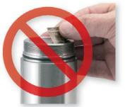
NOTE: Transmitter antenna end caps marked as shown have LEFT-HAND threads. Turn COUNTER-CLOCKWISE to replace.
