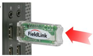
A red LED on the device will flash every three seconds, indicating Configurator is seeking to establish a communication link with a transmitter.\*
