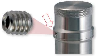
Loosen the set screw in counter-clockwise (CCW) direction with 3/64-in. [1.2 mm] Allen wrench provided with transmitter.
