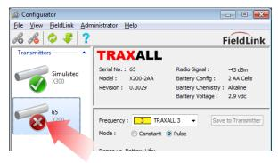
Connection failure can also indicate a system timeout. Upon activation, the transmitter will attempt to establish a communication link.
