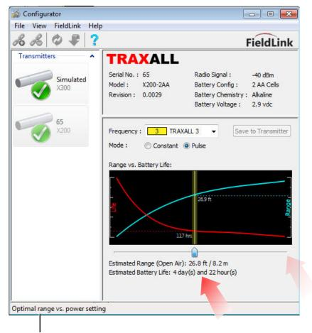
STATUS: OPTIMAL RANGE/POWER BALANCE FOR THIS TRANSMITTER
